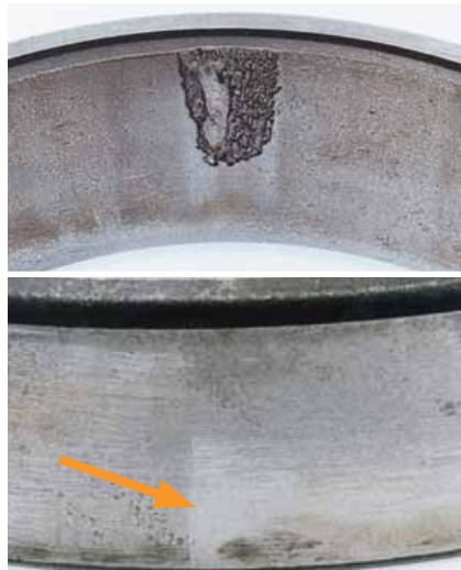
Localized spalling on the cup race from stress riser created by split housing pinch point.
