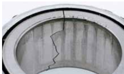
Cone bore damage: Fractured cone due to out-of-round or oversized shaft.
