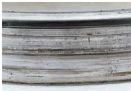
Cup spinning: Loose cup fit in a rotating wheel hub.
