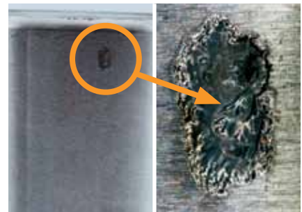
Electric arc pitting: Small burns created by arcs from improper electric grounding while the bearing is stationary.
