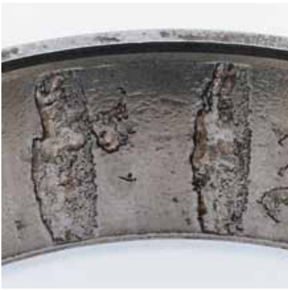
Line spalling: Roller spaced spalling from bearings operating after etching damage.
