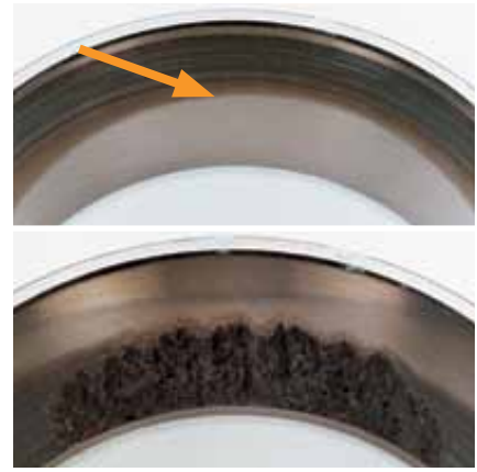
Irregular roller path from deflection, inaccurate machining or wear of bearing seats.
